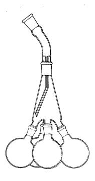
Multiple Flask Receiver— Includes four separate receiver flasks, rotatable so that only one of the flasks receives distillate or residue at a time. Available with 200 ml, 500 ml or 1 liter flasks. Replaces standard receiving flask on still. Utilizing 2 sets allows straightforward mass balance determination and feed rate confirmation.
