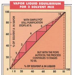
Note that the shape of a vapor composition equilibrium diagram will vary widely with the particular
