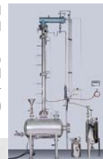
4-gallon, 2" diameter, high vacuum and high temperature Fractional Still for fine chemicals manufacturing
