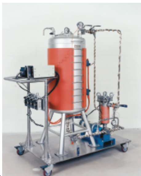
Portable polymer recirculation/dispensing system with heaters and filter vessel.
