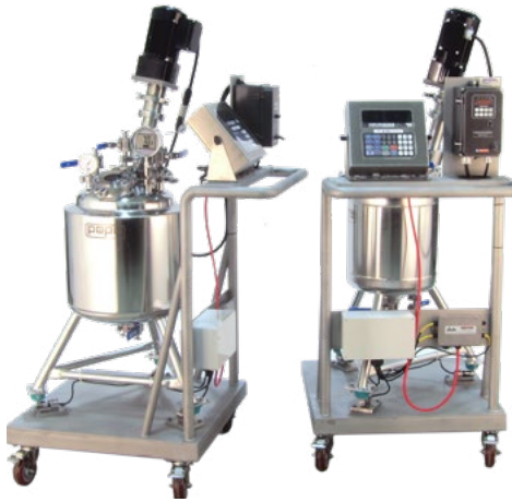
25-L Mixing Vessels with Load Cells, Carts
