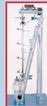
Batch Fractionating System with 2 gallon boiling vessel, 1" column, condenser, all stainless steel.
