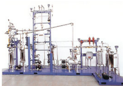
Skid-Mounted Purification Plant, with 2" diameter fractionating column, reboiler, condenser, vaporizers, pumps, control elements, vessels and other components.
