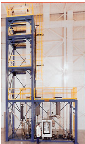
Pope Hybrid Distillation System, incorporating 12" diameter fractionating column with 10-square foot wiped-film evaporator for purification of heat-sensitive compounds. System also incorporates Molecular Still and explosion-proof control system.
