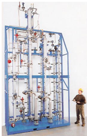
Still Mounted Continuous Purification System with 3" and 4" fractionating columns, plus absorbers, dessicator columns and control elements.
